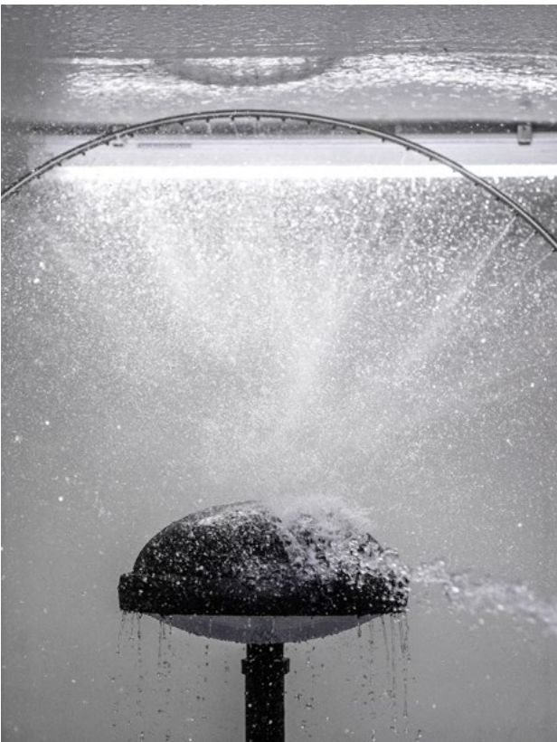
ATP test: projection of water from all angles at an average of 100 l/min with a pressure of 100 kN/m 2 .
