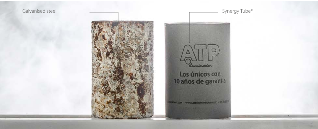
Galvanized steel pole section from another manufacturer and ATP Synergy Tube®, both after 2000 hours of exposure in a salt fog chamber.
