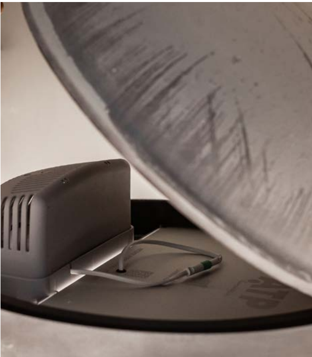
ATP test: continuously moving cloud of 2 kg/m 3 of dust with a diameter of less than 75 µm.
