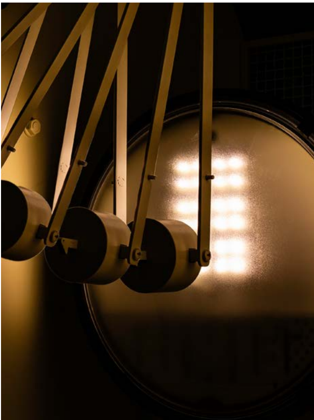
ATP testing: impact of 50 joules of energy with a 5 kg club.
